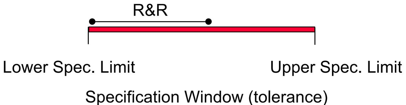
*About 50% of the tolerance, in this example, is used up by the Measurement System variability. This leaves only 50% for the Process variability!*
